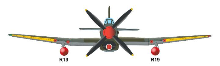
Napalm bomb does not hang centrally beneath the bomb carrier put is offset inwards.
