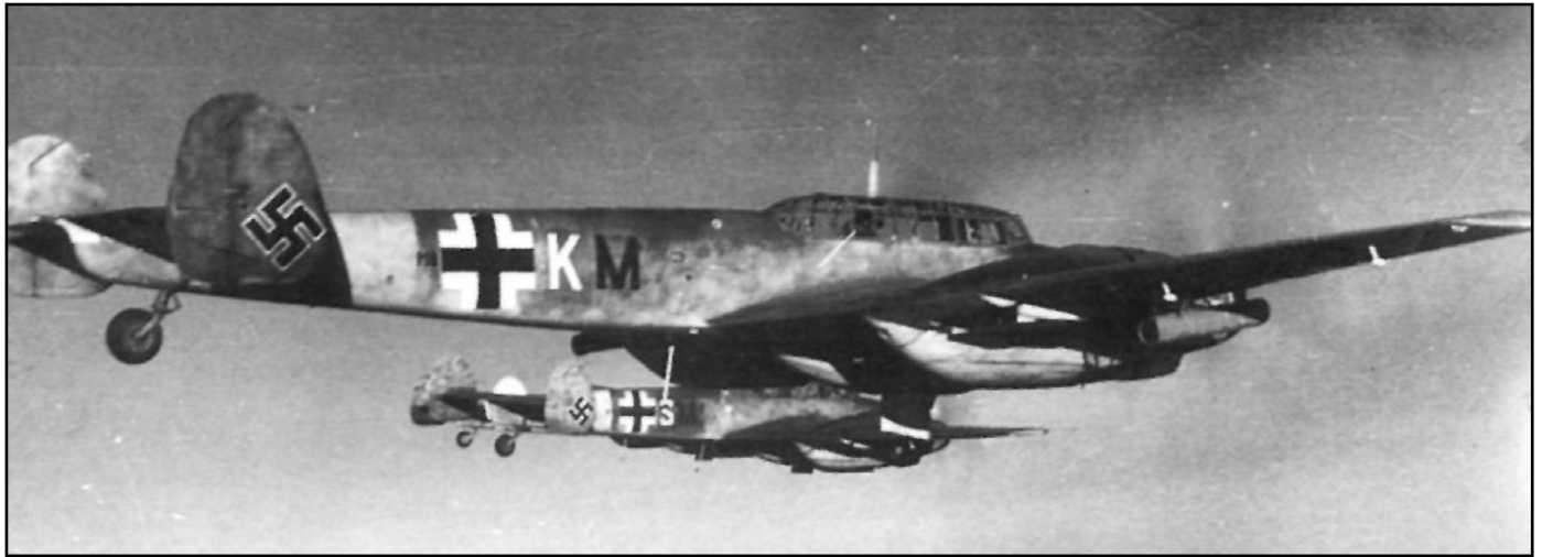
A group of 4. Staffel ZG 76 with Flak 18s. Clearly visible on both birds are the ammo chutes of the Flak 18. The near aircraft M8+KM carries underwing W.Gr.21s, while M8+SM does not.
