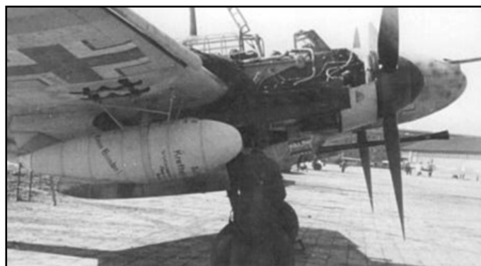
Photograph of another variation on the Bf 110 with the R1 mod, this time with drop tanks.
