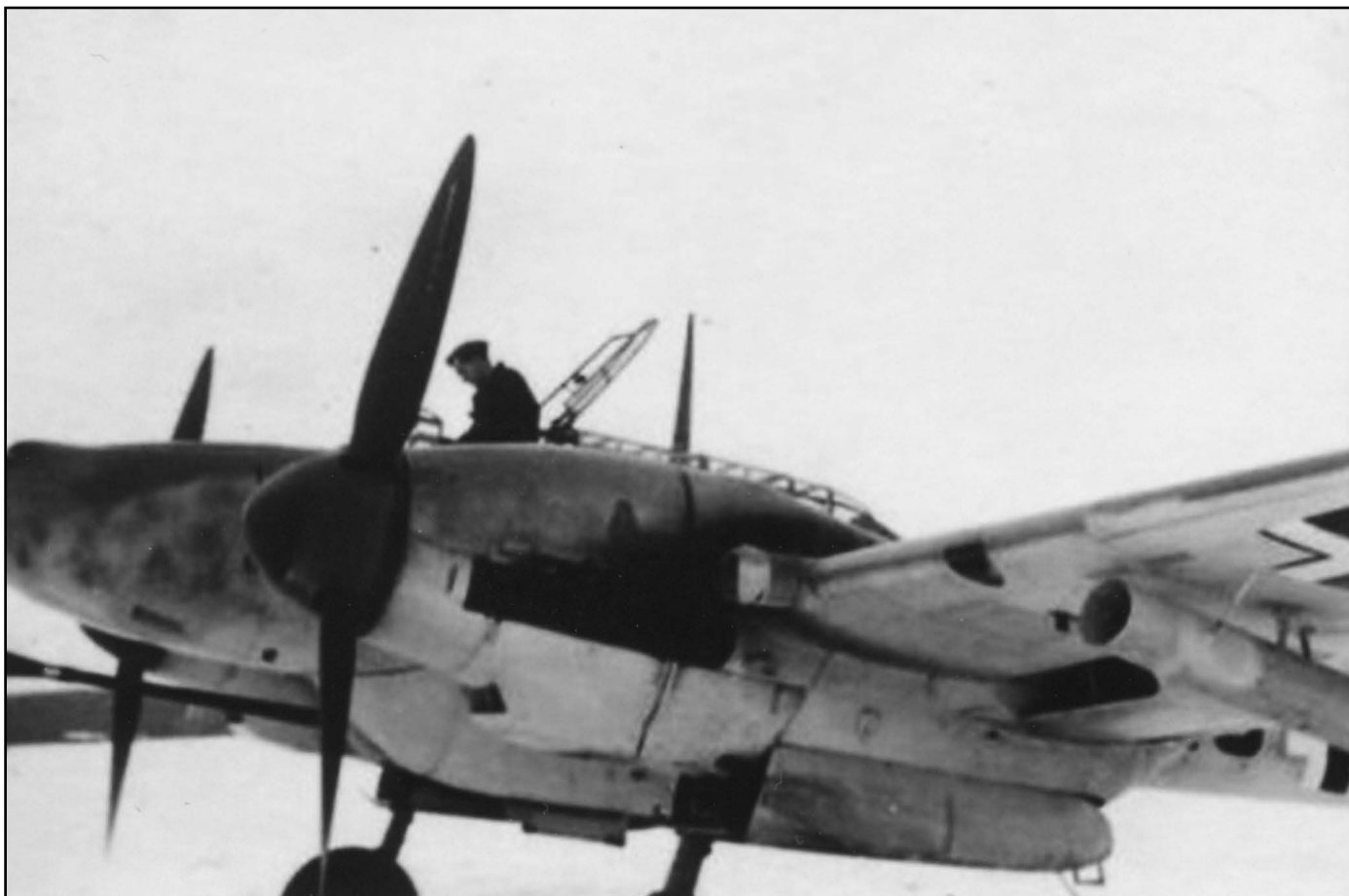
An interesting Bf 110 G; it mounts a filter commonly seen in the dustier regions of the Eastern Front. This aircraft could be dubbed 'Superzerstörer', given that it also can bite with W.Gr.21 underwing rockets along with the Flak 18.
