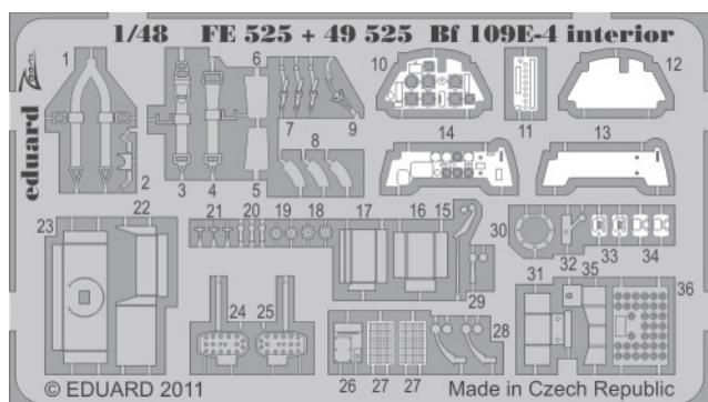
1. Separate the etched components from their frames on the protective paper. Removal from the paper is done only after separation of the parts from the frames.
