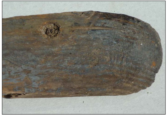
Detail showing the rounded end of the wooden frame. It is worth noting the remains of the RLM 75 color, with which the entire frame was painted. This artifact does not come from aircraft W.Nr. 681456 flown by Uffz. Eilmes, unlike the previous pictures of metal frames, but rather from Sturmbock W.Nr. 681355 flown by Uffz. Zuber.
