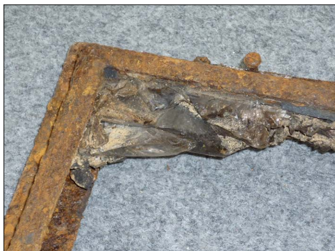
Detail of the remains of armored glass from the lower rear corner of the left side window.
