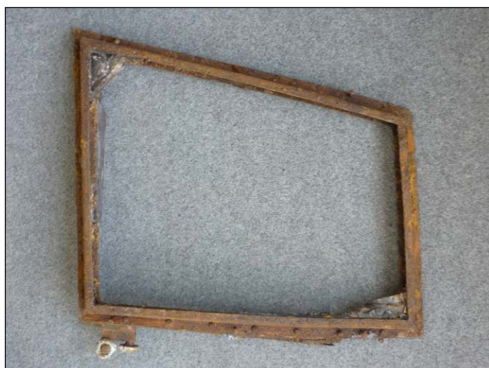
Port side of the glass frame, including the roller mechanism for sliding the canopy.
