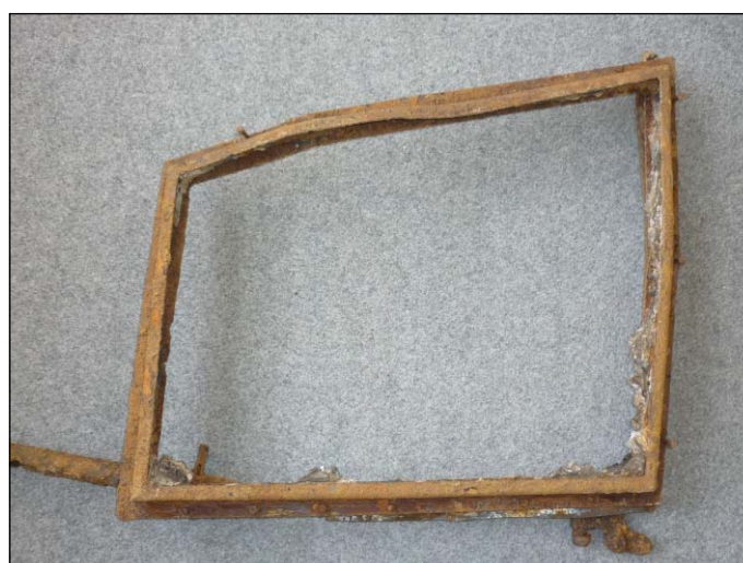
Frame from the starboard side of the canopy. The long segment is part of the tube construction of the cockpit canopy.
