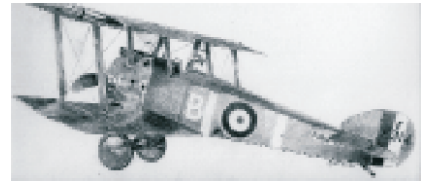
British Sopwith Camel, with Clerget 9B 130 hp engine, max. speed 185 km/h.
