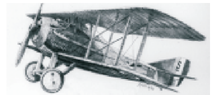
French SPAD XIII, powered by Hispano Suisa 8BEc 235 hp engine, max. speed 220 km/h. USAAC also acquired these aircraft.
