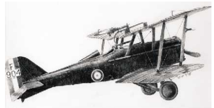
British SE 5a, powered by Wolseley W.4A Viper 200 hp engine, max. speed 222 km/h
